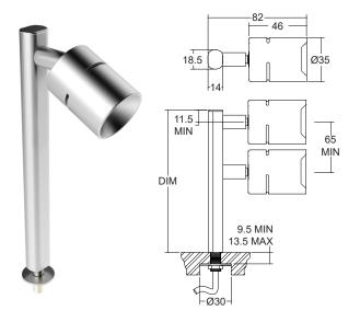
Method 2 - surface mounted option with cable exit at the back. Specify stem length, number of spotlights and spacing.
